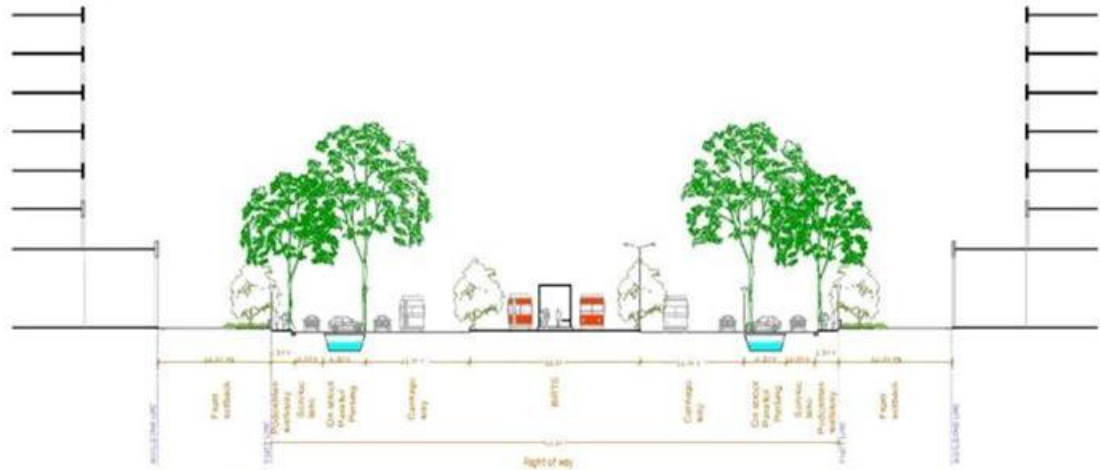
PROPOSED SECTION for 60 MTS WIDE ROAD WITH BRTS(NH)
