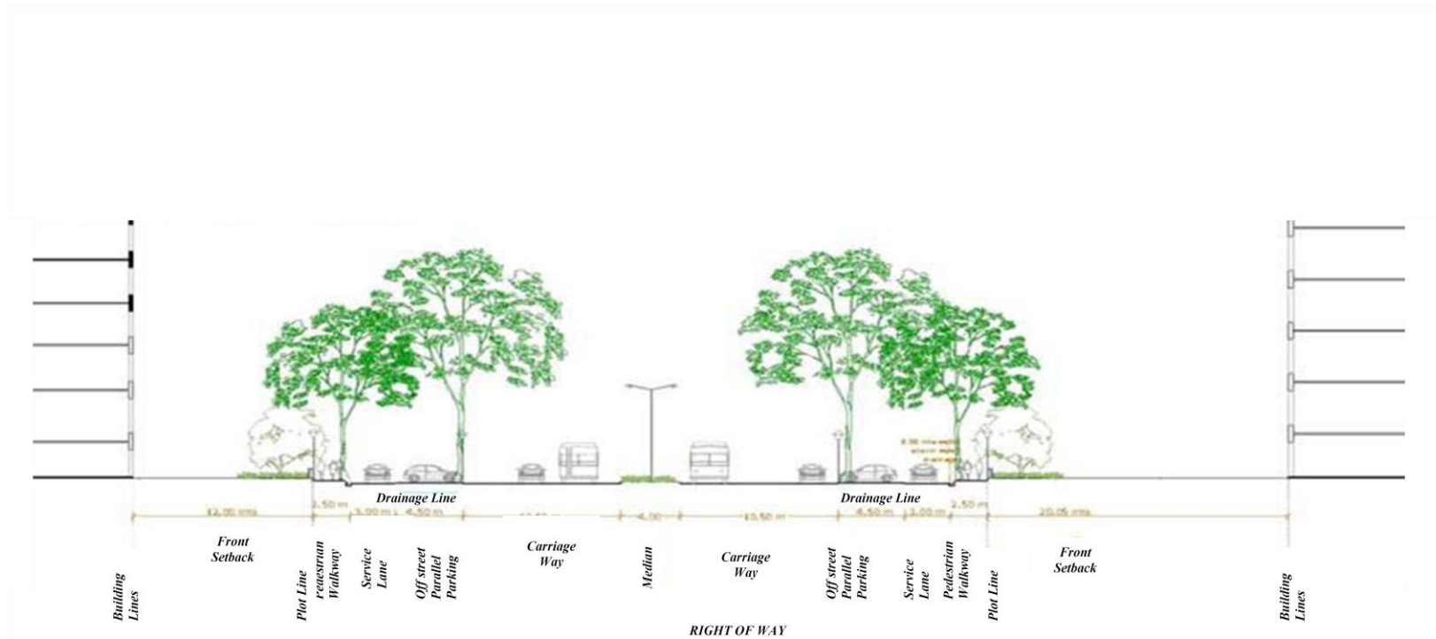
Figure 9: Pocket Major Road (45 meter wide) - Road Section
